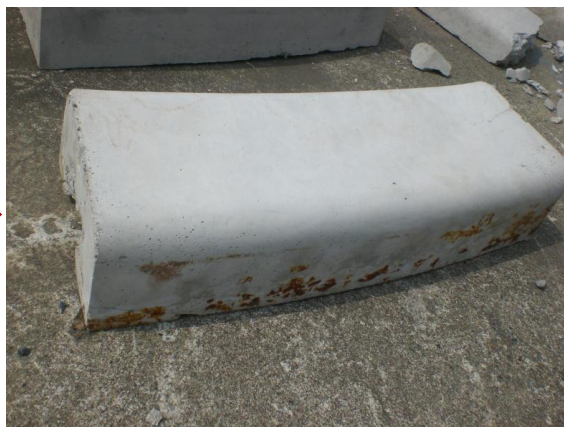
Red-rust on the mold transferred to the product
